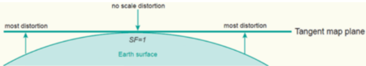
Scale distortions on a tangent map surface. The central point is not distorted on the map
